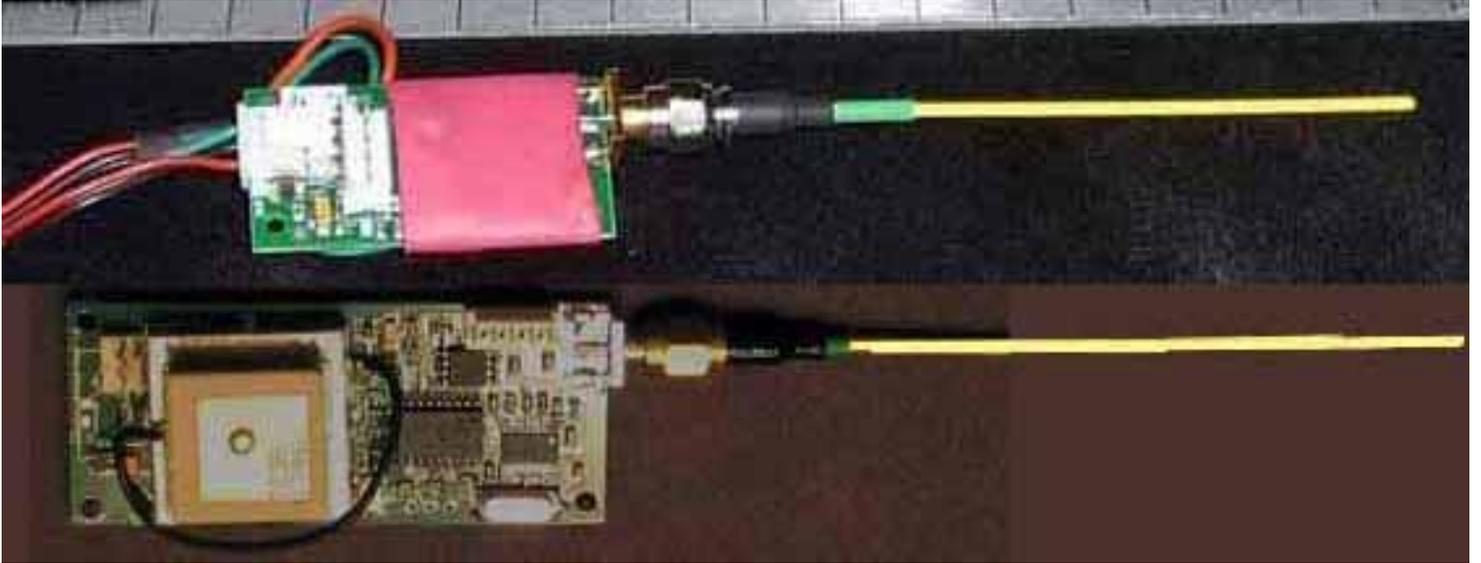
We are looking for a ride on one or more rockets at the Austin Area Rocketry Group's October 2 launch. These flights will be used to test our rocket tracking system described below. Our payload is pictured above (full size, cm ruler) and consists of two small radio transmitters having a mass of about 30 and 60 grams.
